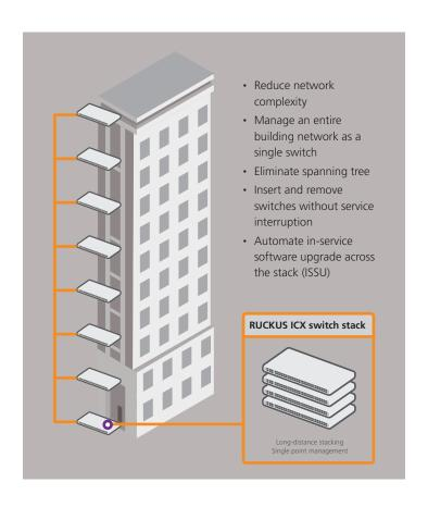
Some ICX switches, like the ICX 7150-48ZP and ICX 7650-48ZP models, take PoE to the next level with support for the 802.3bt standard (pending ratification) delivering up to 90 watts per port to support power-hungry PoE devices such as next-generation wireless access points, large video displays, pan/tilt/zoom surveillance cameras and other devices.
