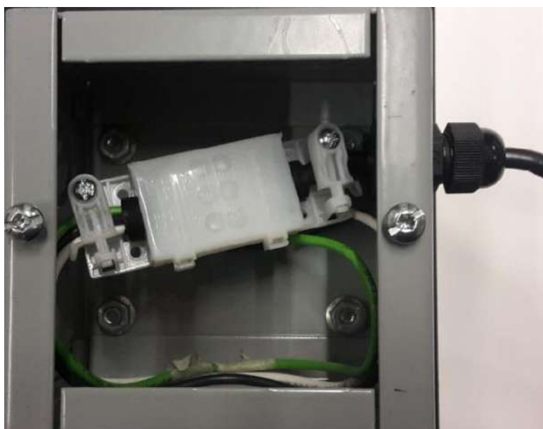
Fig. 43 Completed electrical connections to the projector 74-00013-01
